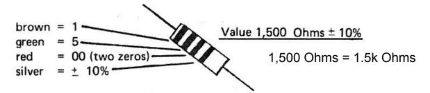
Give the value in Ohms and the Tolerance of the following resistors.
