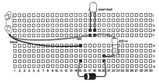
**Step 2 -** Install the DIODE with the CATHODE lead into hole 15b and the ANODE into hole 20b.
