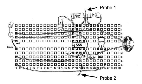
Step 3 - Connect the battery to the Battery Snap. You can experiment by putting the Probes into water and hear the tone from the speaker.
