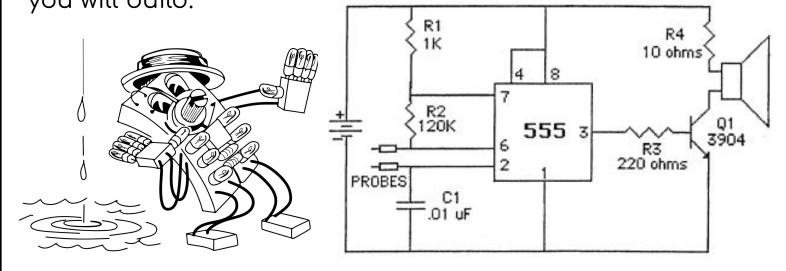
This circuit uses a 555 Integrated Circuit as **CLOCK**. Pin 3 emits a **signal** to the speaker.
