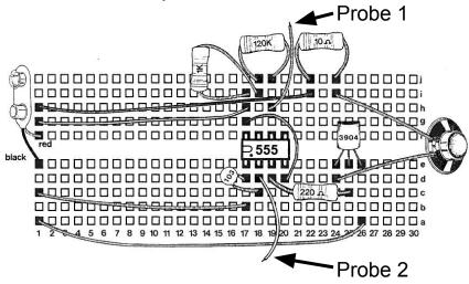
Step 2 - Install all the parts on the SCB as shown above.
